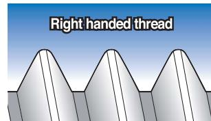
A thread which, when viewed axially, winds in a clockwise and receding direction. Threads are always right handed unless they are specified
